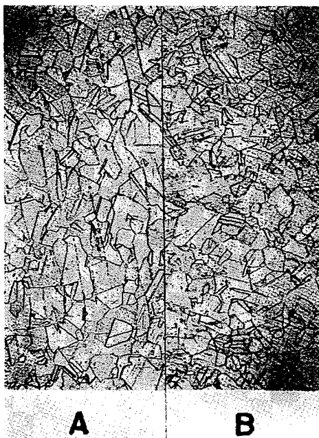
FIG. 1, A. Photomicrograph \times 100 typical of samples 1, 2, and 3 cut from bar stock. FIG. 1, B. Photomicrograph \times 100 of sample cut from rod stock.
